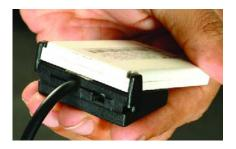
Attach the clip in place of the battery, so that the pins of the clip touch the point provided on the base.
