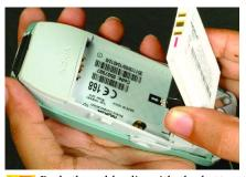
Push the cable clip with the battery in the slot until it clicks into place. Attach the other end of the cable to the serial or USB port of your PC.
